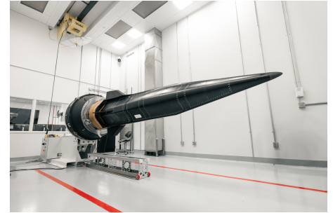
The "That's Not A Knife" mission payload: DART AE, a scramjet-powered aircraft developed by Australian aerospace engineering firm Hypersonix.
