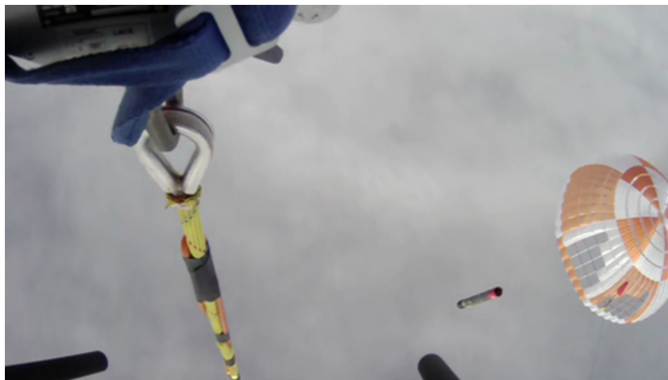
View from recovery helicopter of Electron booster returning to Earth under parachute after launch (Photo: Business Wire)
